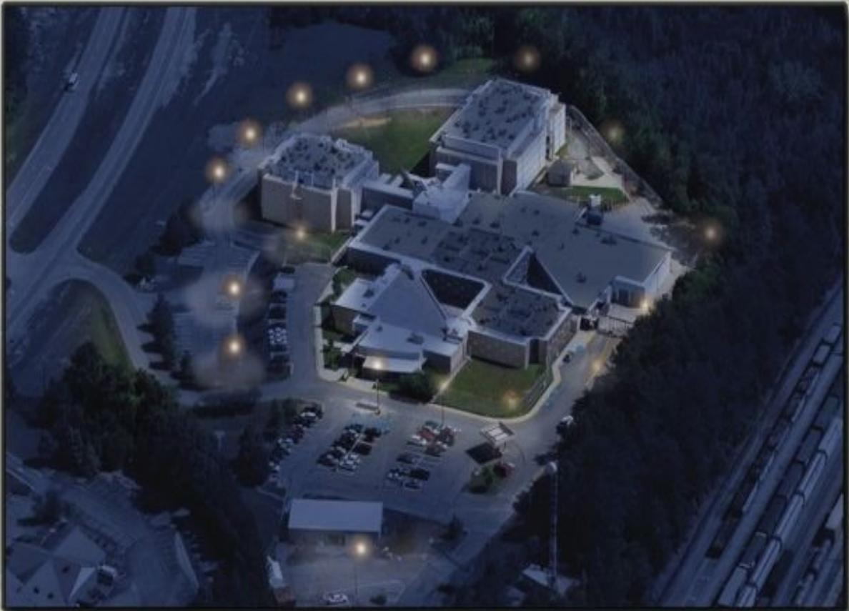
Perimeter Security lighting assessments conducted recently indicate a critical need for additional exterior security lighting at the Jail. Recommendations calls for a level - 5 enhancement, which will require replacement of our existing outdoor High Pressure Sodium Lighting Fixtures and Directional Flood Lights with new LED Galleon Fixtures.
