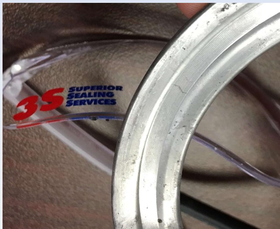
Laboratory Testing – Gasket Analysis After Testing
