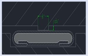
Un-Compressed DMJ Gasket. The Nubbin should sit in the center of the gaskets cross section
