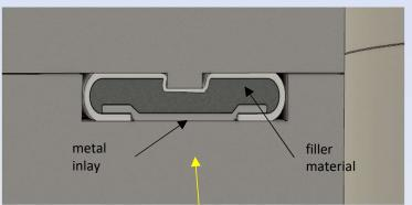
Even though the nubbin creates a high stress point on one side of the gasket there is still large surface area contact (metal to metal) after gasket compression.
