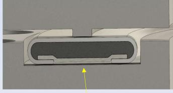
When load is applied to the gasket the nubbin will compress into the flat of the DMJ cross section in turn pushing the metal inlay through filler (e.g. graphite – PTFE) densification to the groove base.
