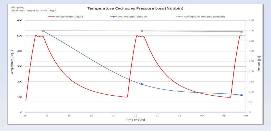
The above table outlines the remaining gasket stress after two temperature cycles. Even though the DMJ gasket lost significantly more internal pressure in the test this was not due to low gasket load.
