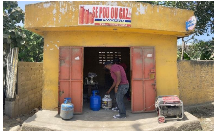
Fig. 2. A propane refilling station in Cap-Haïtien, the sign translates to “it’s for you gas.” This station used a gasoline generator to operate its propane pump (July 2023)
