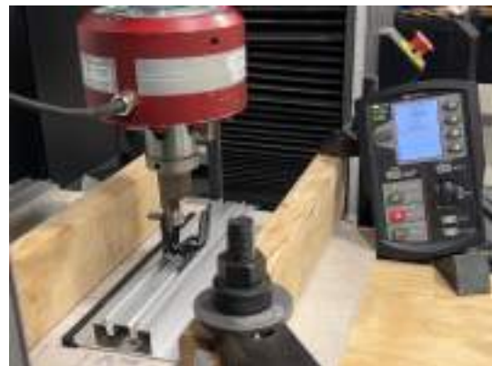
Photo 4: Approximate load before bolt slipped, 520 lbf
