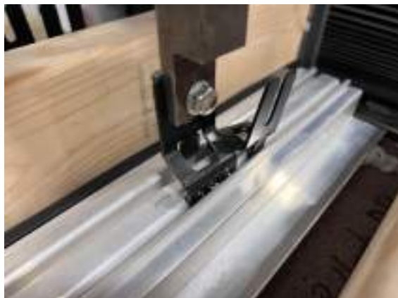
Photo 5: "H" bracket deformed and slipped out of Multiballast DB base test #1
