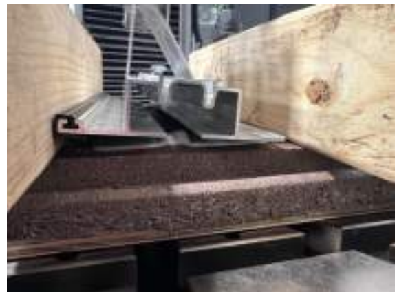
Photo 12: Tension test #4 adhesive failure, aluminum to adhesive
