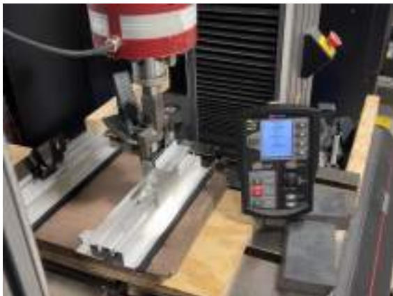
Photo 15: Compression test #1 near max load before tile broke
