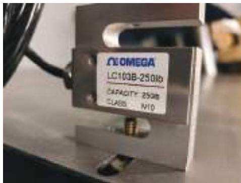
Figure 5: Load Cell Model used for tests
