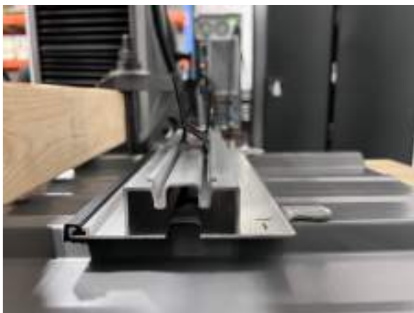
Photo 5: Tension test #1 "H" bracket slipped out
