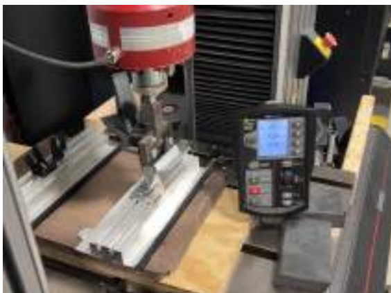
Photo 17: Compression test #2, permanent deformation visible
