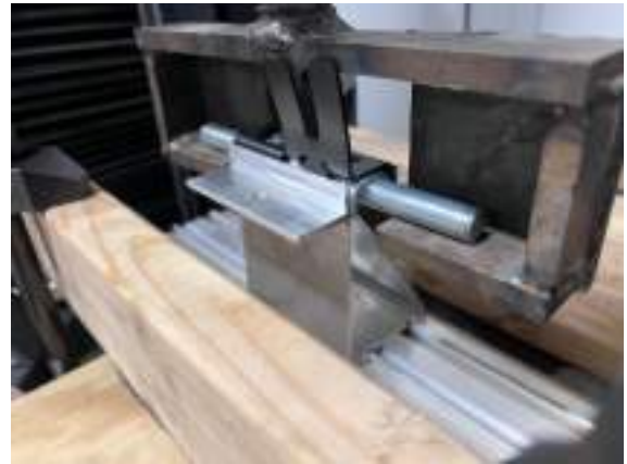
Photo 8: Tension test setup with riser bracket
