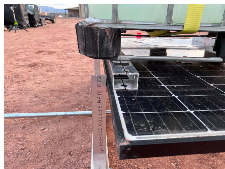
PHOTO 8: Slight deflection noted under load
