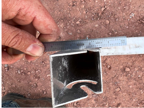
PHOTO 11: Slight deformation after load removed
