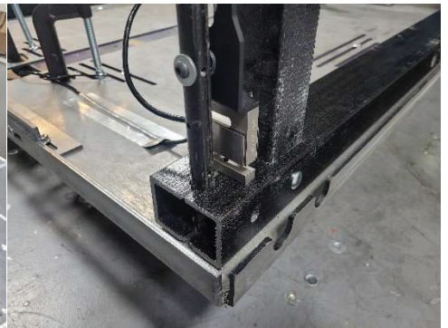
Figure 15: Load cell location at leading edge, LC0-1 & LC0-2
