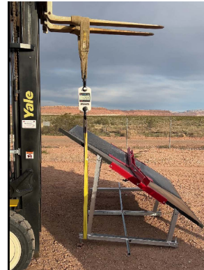
PHOTO 2: Test setup under max load
