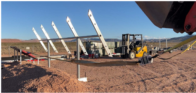
PHOTO 1: Horizontal force test setup
