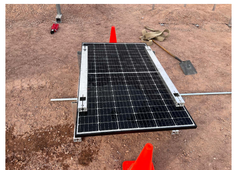
PHOTO 9: IR-30 system after compressive load tests
