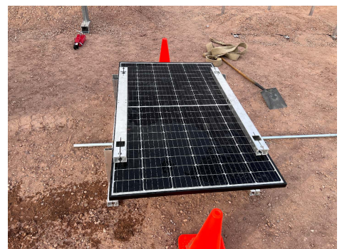
PHOTO 9: IR-30 system after compressive load tests
