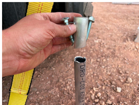
PHOTO 8: Second anchor - second test where anchor failed at drilled thru hole
