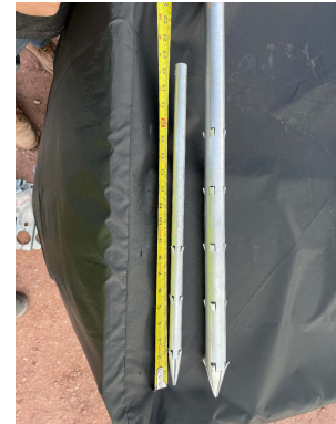
PHOTO 3: AnchorSpikes. The small AnchorSpike was used for setup in this test
