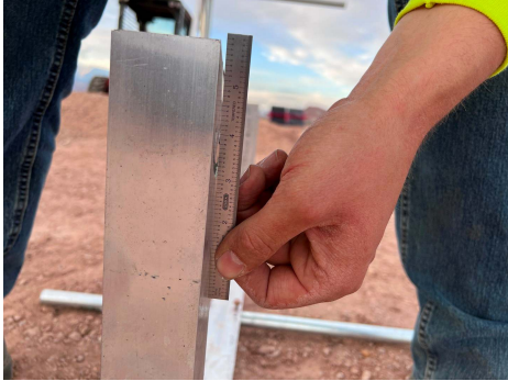
PHOTO 10: Slight deformation after load removed
