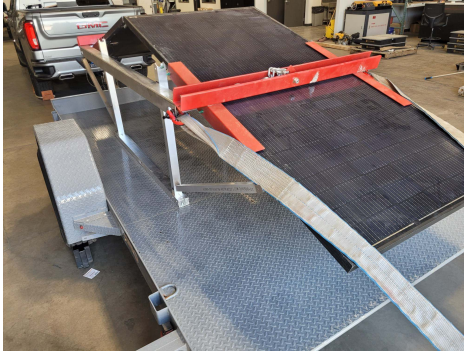
Photo 1: IR-EW15 BallastRack with 2 solar panels installed and load application frames (red)
