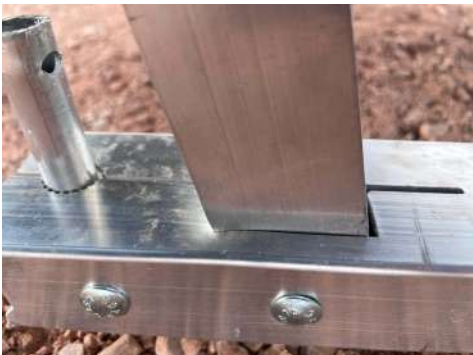
PHOTO 15: Upright deformation after testing
