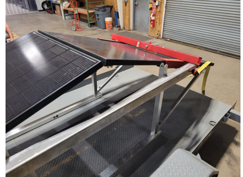
Photo 3: IR-EW15 BallastRack with 2 solar panels installed and load application frames (red)
