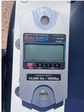
PHOTO 1: Dynamometer used to record loads
