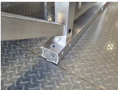
Photo 7: IR-EW15 frame bolted down to hold frame in place for test
