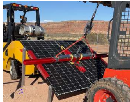
PHOTO 5: Test 1 - Evidence of ballast shift
