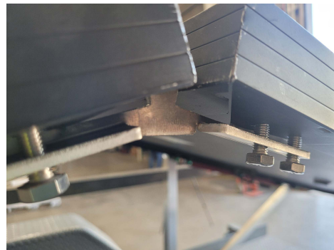
Photo 15: Underside solar panel at top ridgeline after 1500 lbf test load. Solar panel has started deforming at bolts and lifting off the attachment
