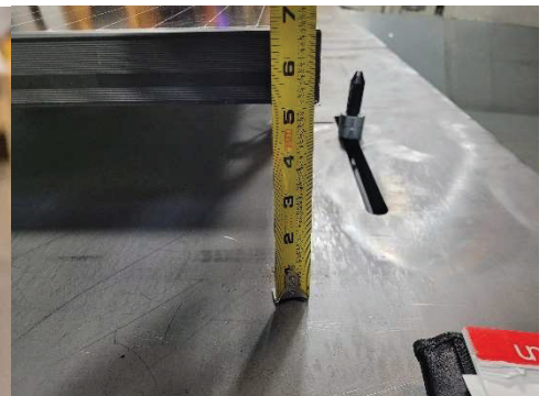
Figure 6: Height from roof to panel, Runs 2 & 3
