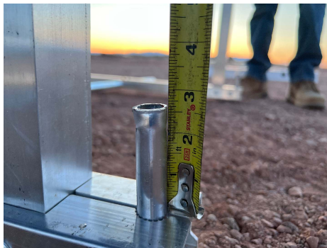
PHOTO 4: 'Stickout' measurement example at Spike #3
