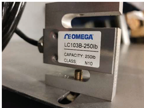
Figure 5: Load Cell Model used for tests
