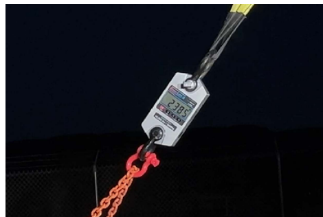
PHOTO 8: Closeup of max load, 2385 lbf
