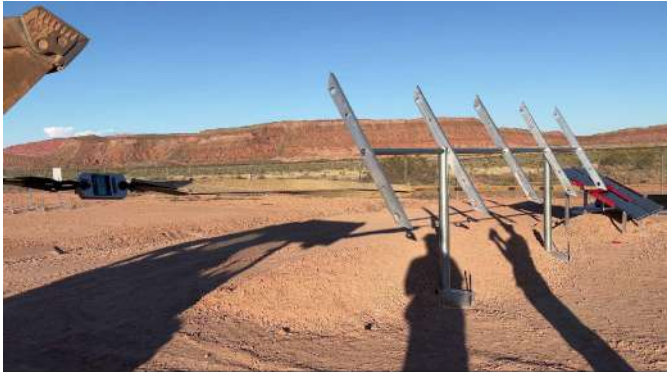
Photo 4: Horizontal force test at max load
