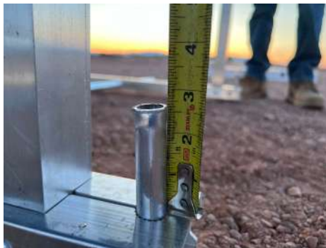
PHOTO 4: 'Stickout' measurement example at Spike #3
