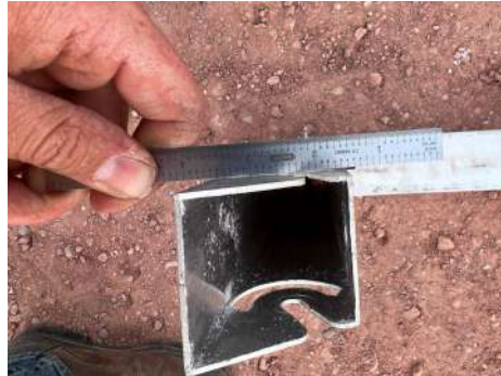
PHOTO 11: Slight deformation after load removed
