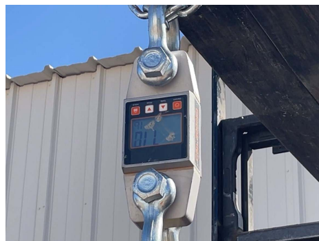
PHOTO 6: Dynamometer scale under load
