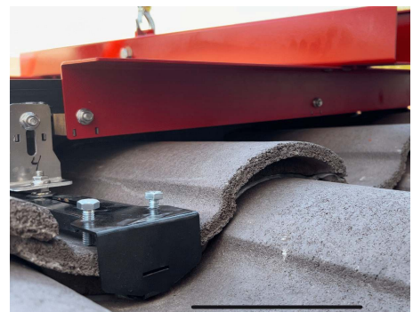
PHOTO 7: Bracket under test load
