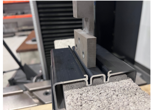
Photo 10: Compression test #3 post test
