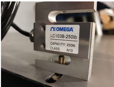
Figure 5: Load Cell Model used for tests
