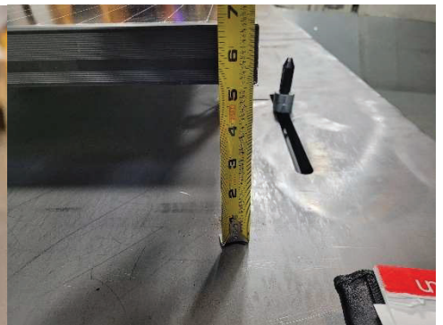
Figure 6: Height from roof to panel, Runs 2 & 3
