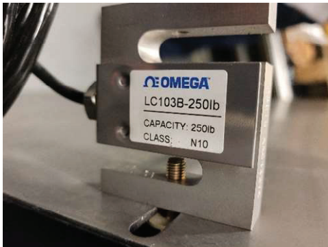
Figure 5: Load Cell Model used for tests
