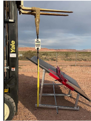
PHOTO 2: Test setup under max load
