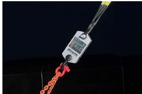
PHOTO 8: Closeup of max load, 2385 lbf
