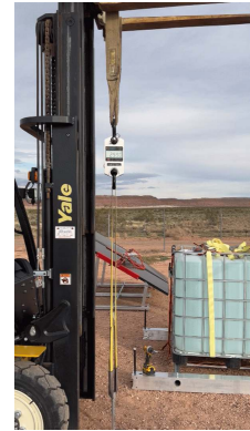
PHOTO 3: Second anchor under load
