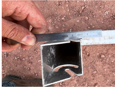
PHOTO 11: Slight deformation after load removed
