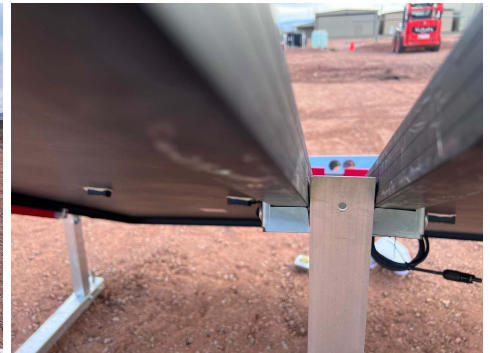
PHOTO 12: Middle brackets after testing
