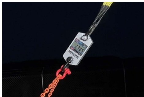
PHOTO 8: Closeup of max load, 2385 lbf
