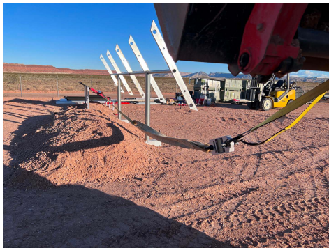
PHOTO 3: Horizontal force test setup
