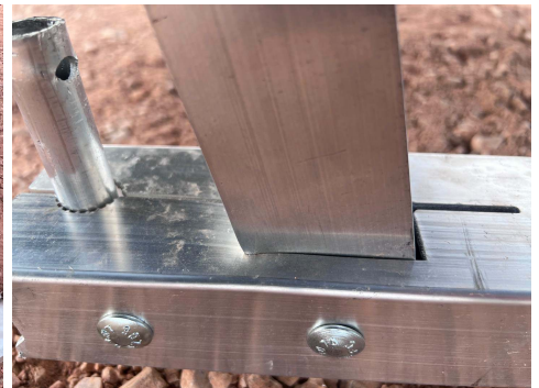
PHOTO 15: Upright deformation after testing
