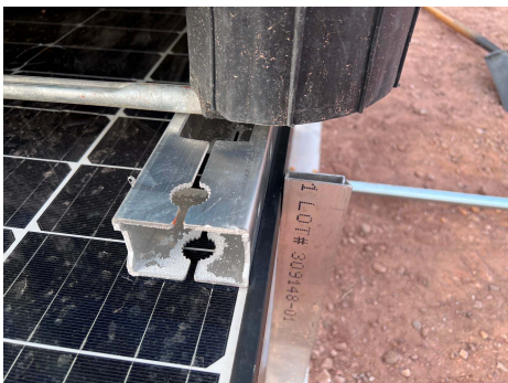
PHOTO 7: Slight deflections noted under load
