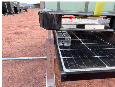
PHOTO 8: Slight deflection noted under load
