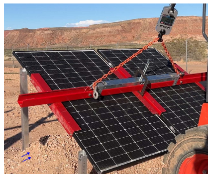
PHOTO 8: Test 2 - Evidence of ballast shift
