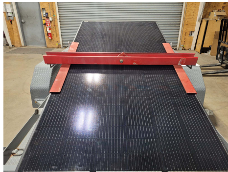
Photo 5: Load point attachment frame on solar panel
