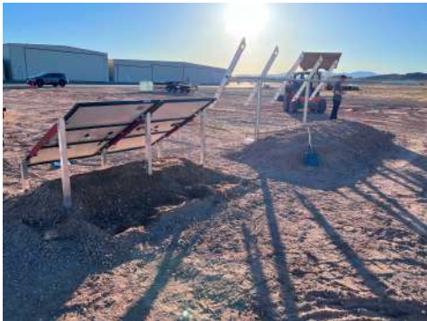
PHOTO 2: Horizontal force test setup
