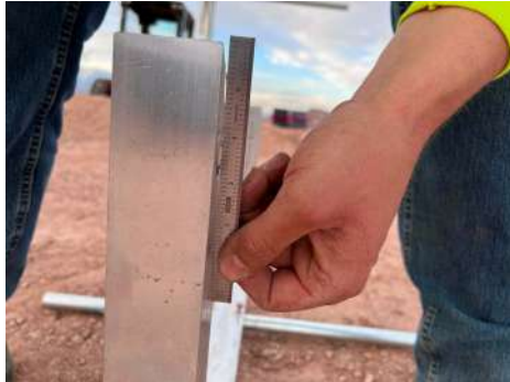
PHOTO 10: Slight deformation after load removed
