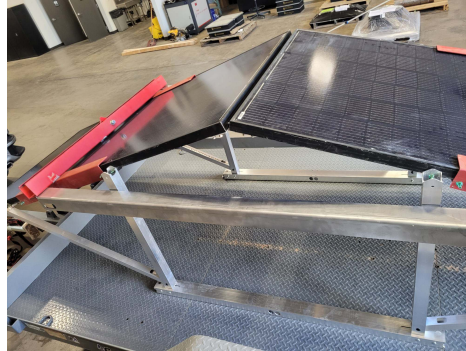
Photo 2: IR-EW15 BallastRack with 2 solar panels installed and load application frames (red)
