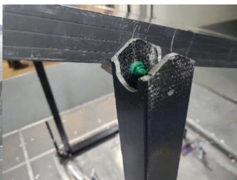
Figure 17: IR Ballast frame connection to solar panel
