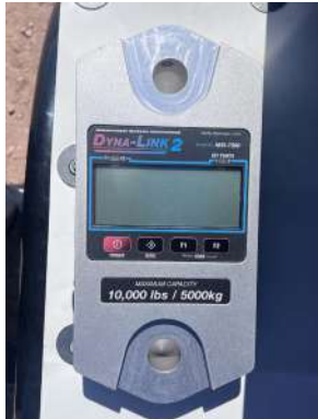
PHOTO 1: Dynamometer used to record loads
