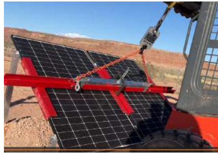
PHOTO 11: Test 2 - Max load
