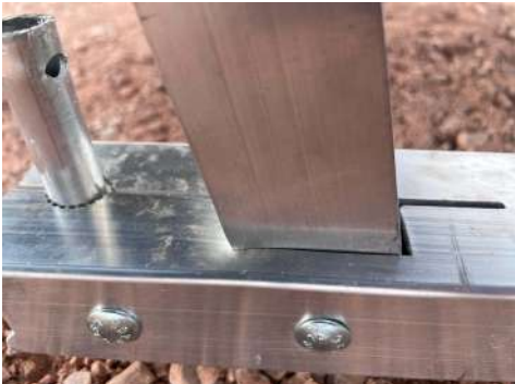
PHOTO 15: Upright deformation after testing
