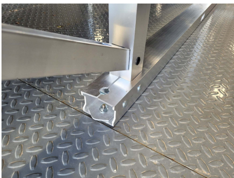
Photo 7: IR-EW15 frame bolted down to hold frame in place for test
