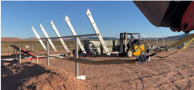
PHOTO 1: Horizontal force test setup
