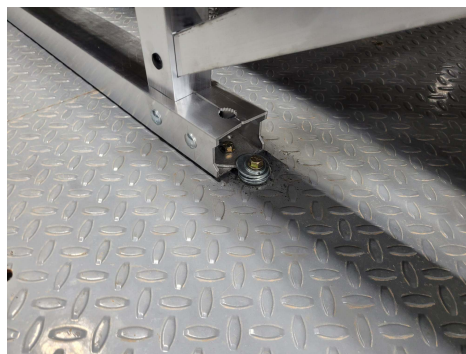
Photo 8: IR-EW15 frame bolted down to hold frame in place for test
