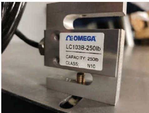
Figure 5: Load Cell Model used for tests
