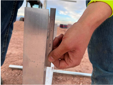
PHOTO 10: Slight deformation after load removed
