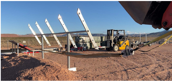
PHOTO 1: Horizontal force test setup
