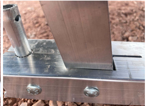
PHOTO 15: Upright deformation after testing
