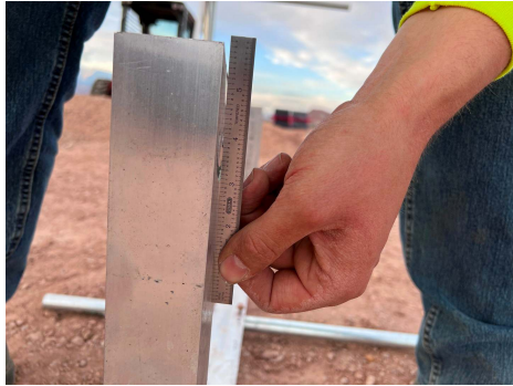
PHOTO 10: Slight deformation after load removed
