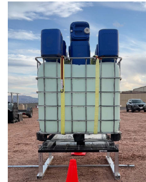
PHOTO 6: Slight deflection under load
