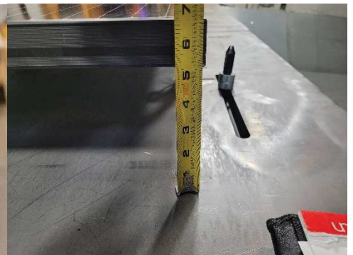
Figure 6: Height from roof to panel, Runs 2 & 3
