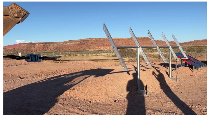
Photo 4: Horizontal force test at max load
