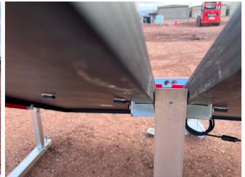
PHOTO 12: Middle brackets after testing
