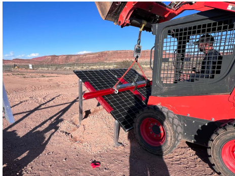
PHOTO 4: Test setup with dynamometer and chains connected
