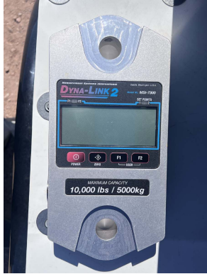
PHOTO 1: Dynamometer used to record loads
