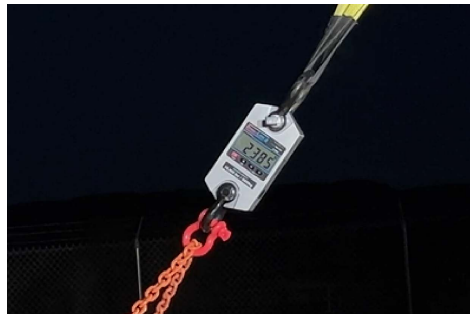
PHOTO 8: Closeup of max load, 2385 lbf
