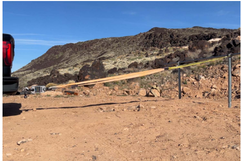
PHOTO 6: Single post test under load
