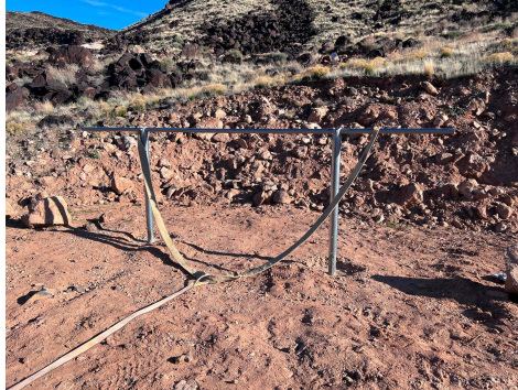
PHOTO 2: Dual post test setup
