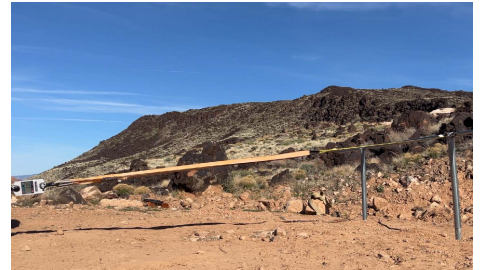
PHOTO 3: Dual post under load
