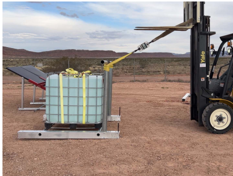
PHOTO 2: Load applied at ~ 45 degree angle
