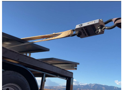
PHOTO 3: Panel under load
