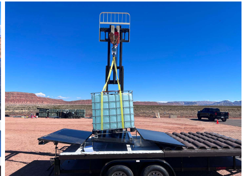
PHOTO 3: Test load being lowered
