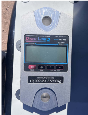
PHOTO 1: Dynamometer used to record loads
