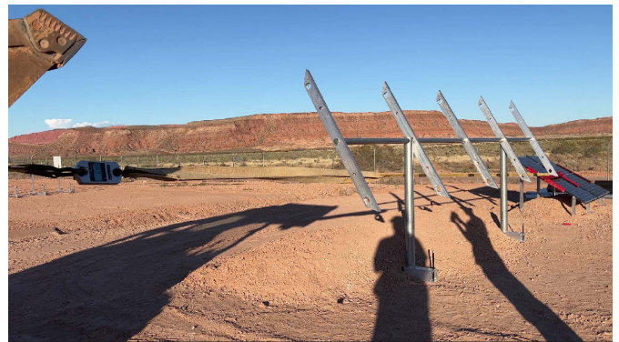
Photo 4: Horizontal force test at max load
