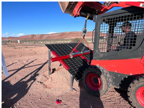
PHOTO 4: Test setup with dynamometer and chains connected
