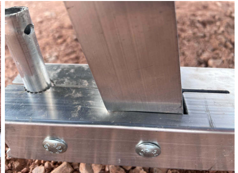
PHOTO 15: Upright deformation after testing
