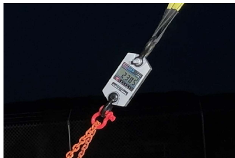
PHOTO 8: Closeup of max load, 2385 lbf
