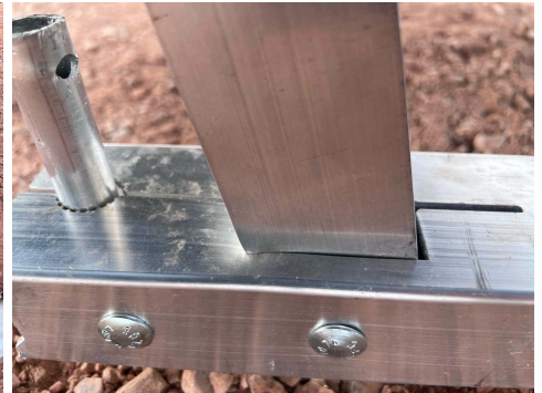
PHOTO 15: Upright deformation after testing
