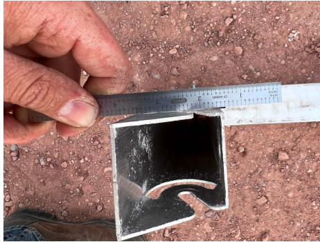
PHOTO 11: Slight deformation after load removed
