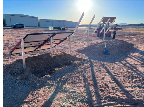
PHOTO 2: Horizontal force test setup
