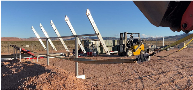
PHOTO 1: Horizontal force test setup
