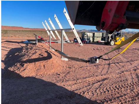
PHOTO 3: Horizontal force test setup
