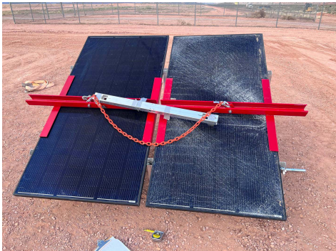
PHOTO 10: Solar panels after testing
