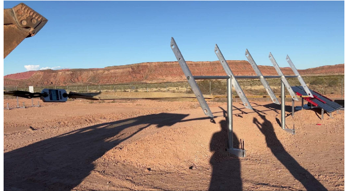
Photo 4: Horizontal force test at max load
