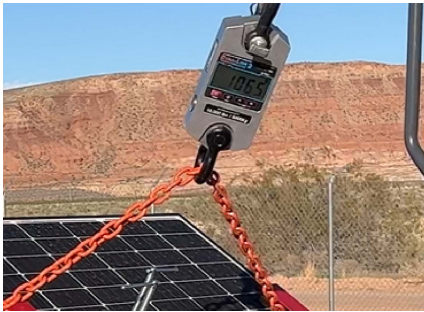
PHOTO 10: Test 2 - Load at ballast shift
