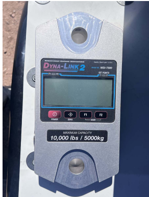
PHOTO 1: Dynamometer used to record loads
