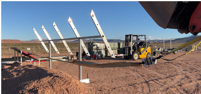
PHOTO 1: Horizontal force test setup
