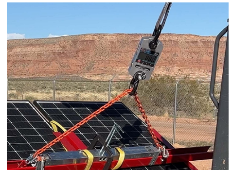
PHOTO 6: Test 1 - Load at ballast shift
