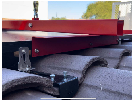
PHOTO 8: Bracket unloaded after test
