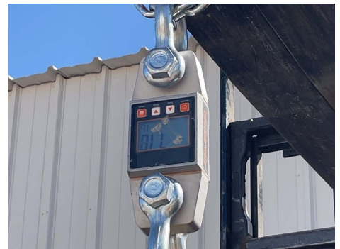
PHOTO 6: Dynamometer scale under load
