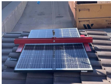
PHOTO 5: Test specimen while under tensile load
