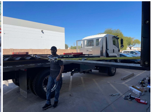
PHOTO 3: Test setup for horizontal pull load
