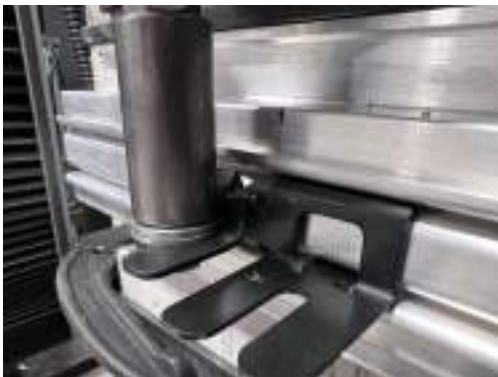
Photo 11: "H" bracket deformation post test
