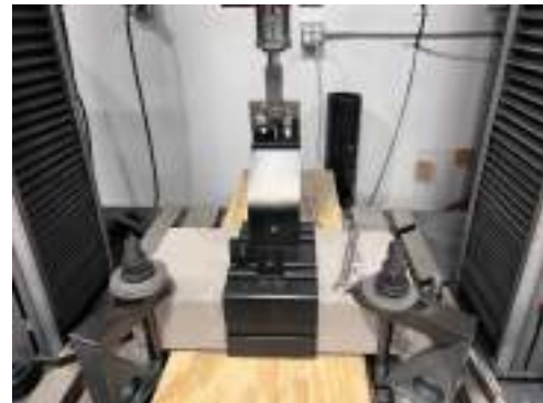
Photo 2: Compression test, setup #1
