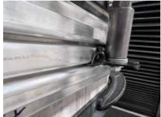
Photo 10: "H" bracket deformation post test
