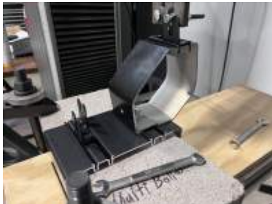
Photo 3: Compression test #1 post test
