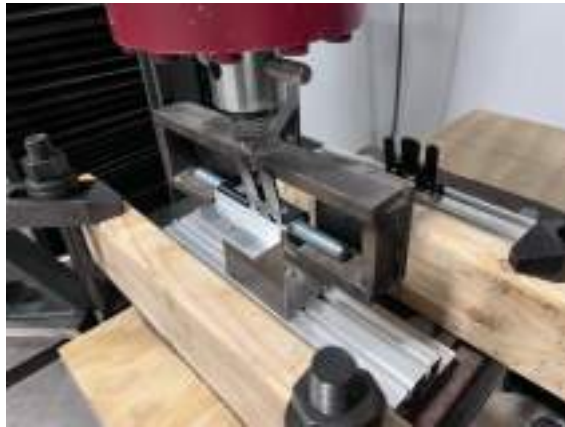
Photo 7: Tension test setup with riser bracket
