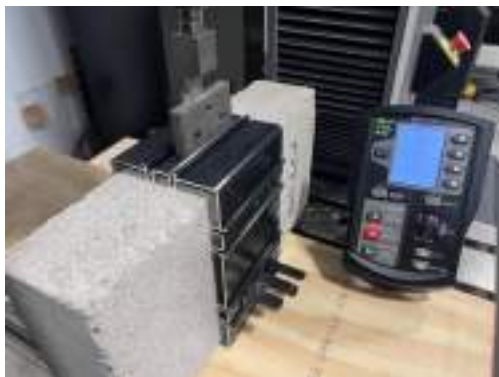
Photo 9: Compression test, setup #3
