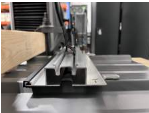
Photo 5: Tension test #1 "H" bracket slipped out
