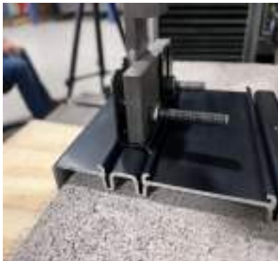
Photo 7: Compression test #2 post test
