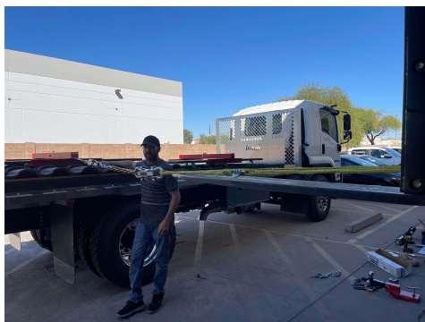
PHOTO 3: Test setup for horizontal pull load
