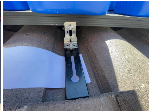
PHOTO 6: Load 2 - Bracket under load
