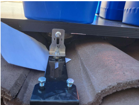
PHOTO 4: Load 1 - Bracket under load
