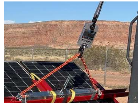
PHOTO 6: Test 1 - Load at ballast shift
