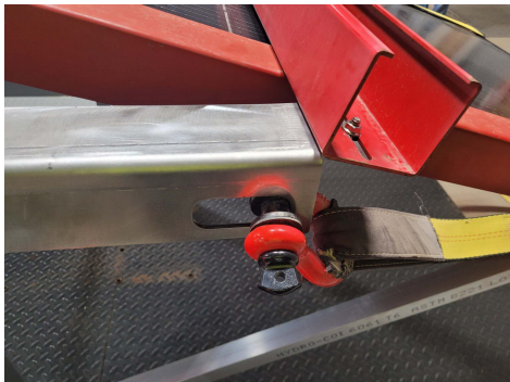
Photo 10: Closeup of load attachment point shackle. The shackle applies load to the tube steel, the tube steel applies load to the red load frame that applies the load to the solar panels.
