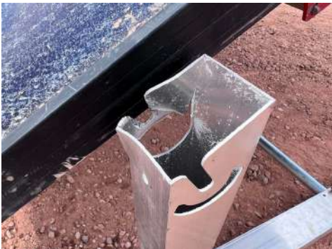
PHOTO 14: Upright mount deformation after testing
