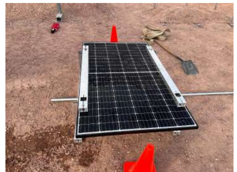
PHOTO 9: IR-30 system after compressive load tests
