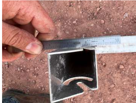
PHOTO 11: Slight deformation after load removed
