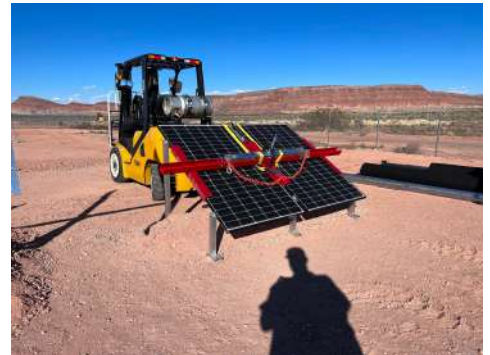
PHOTO 3: Test setup - IR-30 Solar Racking System with red test cross frame
