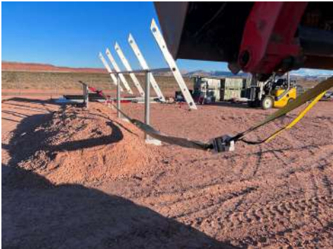
PHOTO 3: Horizontal force test setup
