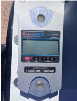
PHOTO 1: Dynamometer used to record loads
