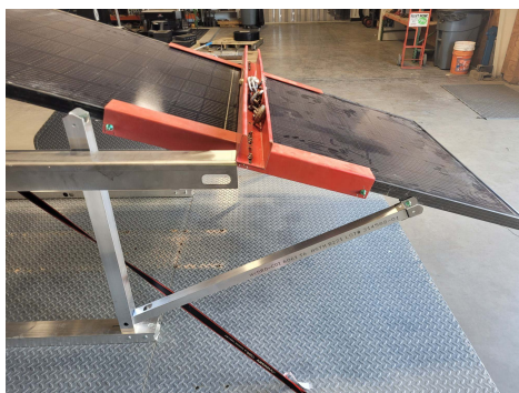
Photo 17: Top of solar panel and system after 1500 lbf test load. No deformation of the IR load frame was observed.
