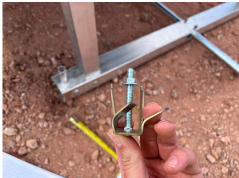
PHOTO 13: Bracket deformation after testing
