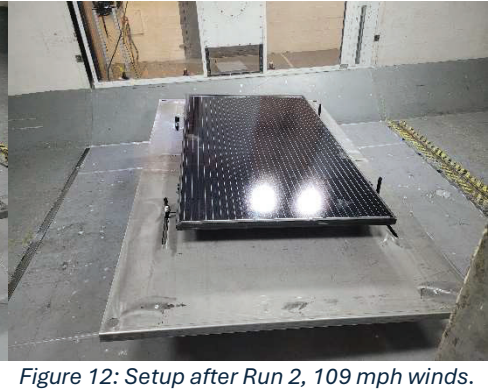
Figure 11: Setup after Run 2, 109 mph winds. No damages or loose hardware noted.
