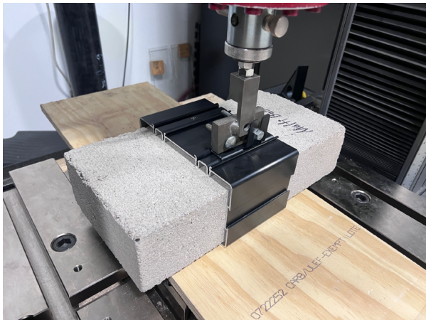
Photo 5: Compression test, setup #2
