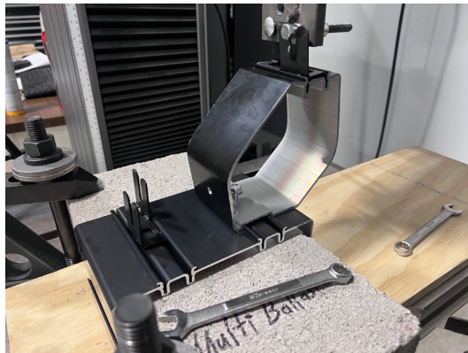
Photo 3: Compression test #1 post test
