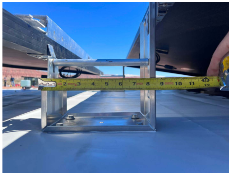
PHOTO 5: Bracket before load
