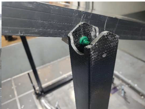
Figure 17: IR Ballast frame connection to solar panel
