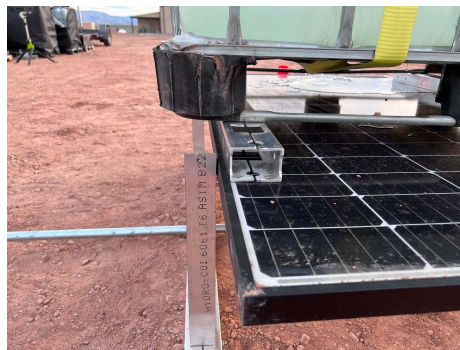
PHOTO 8: Slight deflection noted under load
