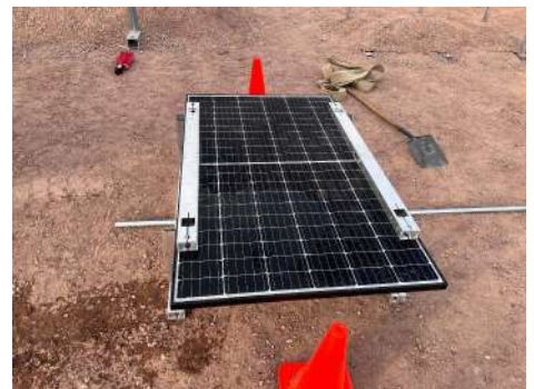
PHOTO 9: IR-30 system after compressive load tests
