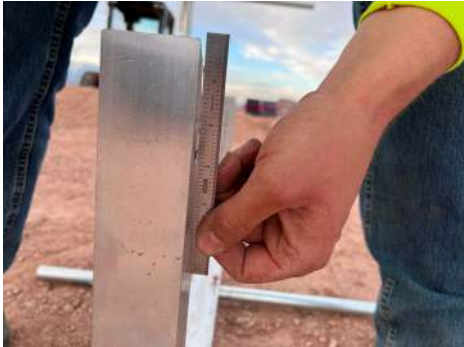
PHOTO 10: Slight deformation after load removed
