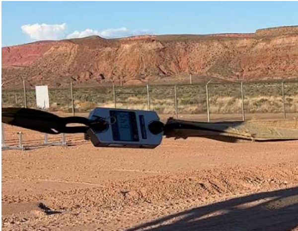
Photo 4: Horizontal force test max load
