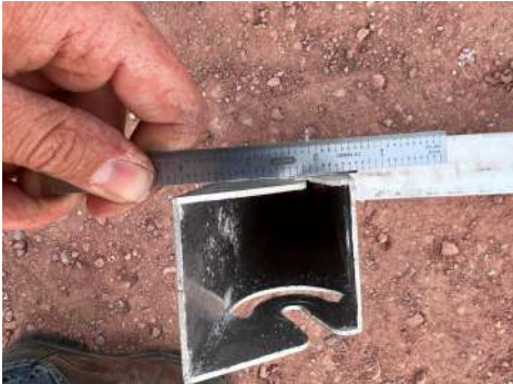
PHOTO 11: Slight deformation after load removed
