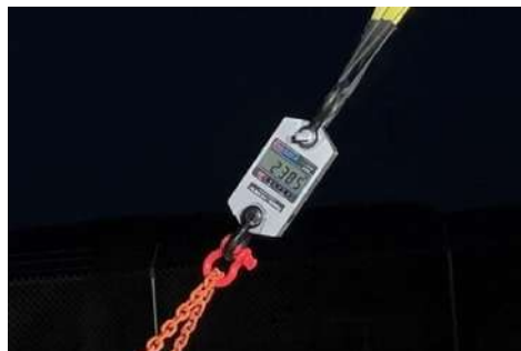
PHOTO 8: Closeup of max load, 2385 lbf
