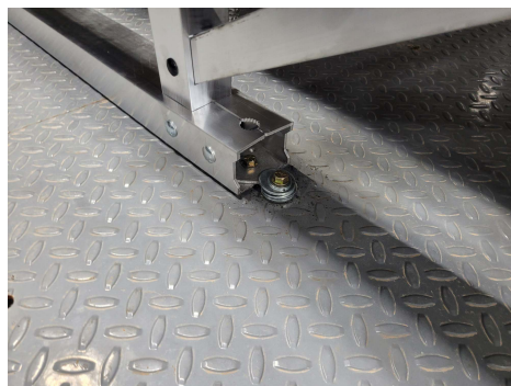
Photo 8: IR-EW15 frame bolted down to hold frame in place for test
