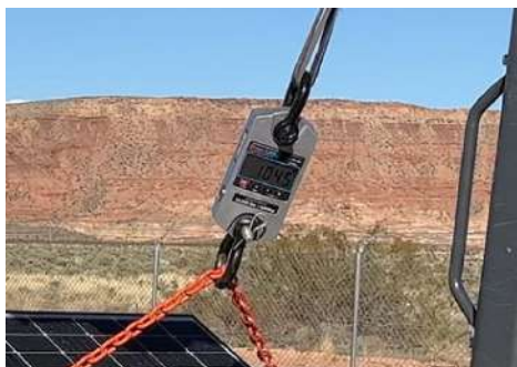
PHOTO 7: Test 1 - Max load
