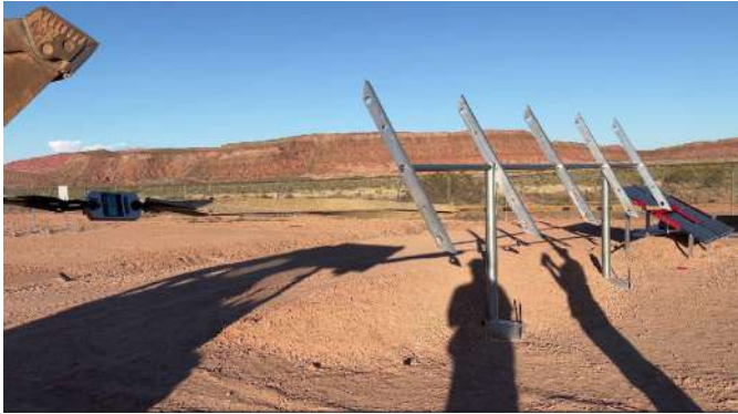
Photo 4: Horizontal force test at max load
