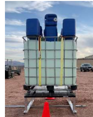
PHOTO 6: Slight deflection under load
