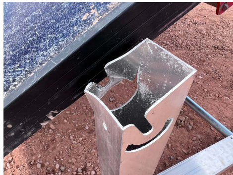
PHOTO 14: Upright mount deformation after testing
