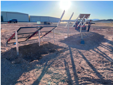
PHOTO 2: Horizontal force test setup
