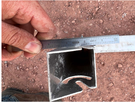
PHOTO 11: Slight deformation after load removed
