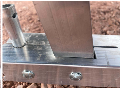
PHOTO 15: Upright deformation after testing
