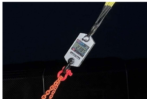
PHOTO 8: Closeup of max load, 2385 lbf
