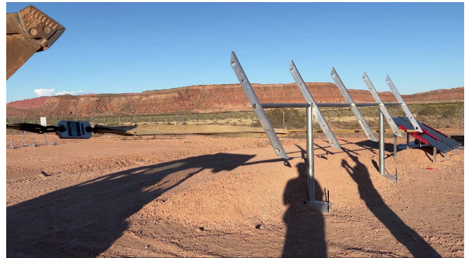
Photo 4: Horizontal force test at max load
