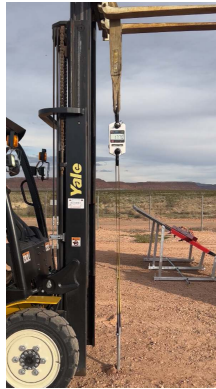
PHOTO 2: First anchor under load
