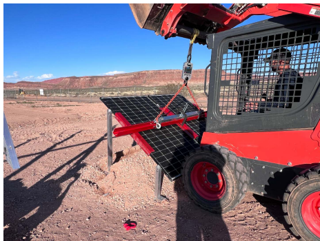
PHOTO 4: Test setup with dynamometer and chains connected
