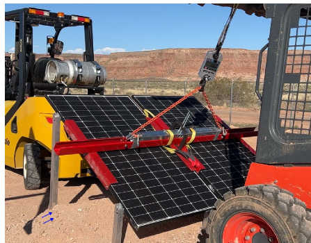
PHOTO 5: Test 1 - Evidence of ballast shift
