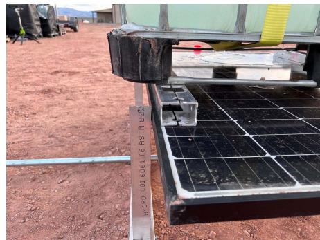
PHOTO 8: Slight deflection noted under load
