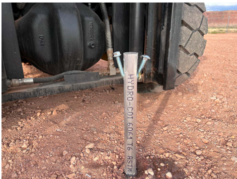
PHOTO 7: Second anchor - first pull where the thru bolt bent and load strap slipped off
