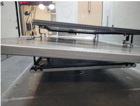
Figure 13: Setup after Run 2, 109 mph winds. No damages or loose hardware noted
