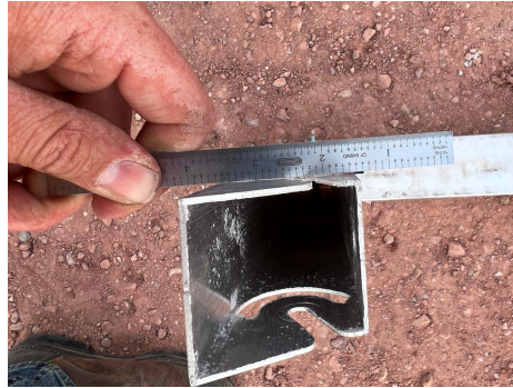
PHOTO 11: Slight deformation after load removed
