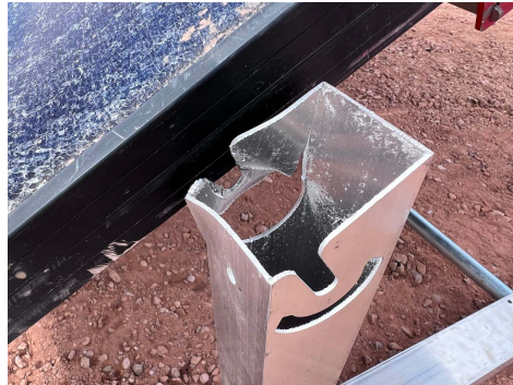
PHOTO 14: Upright mount deformation after testing
