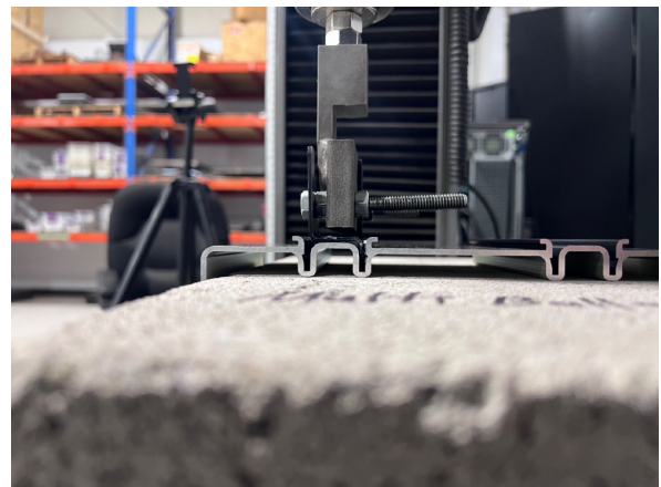
Photo 6: Compression test, setup #2
