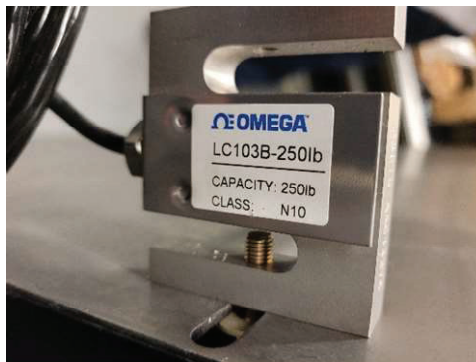
Figure 5: Load Cell Model used for tests
