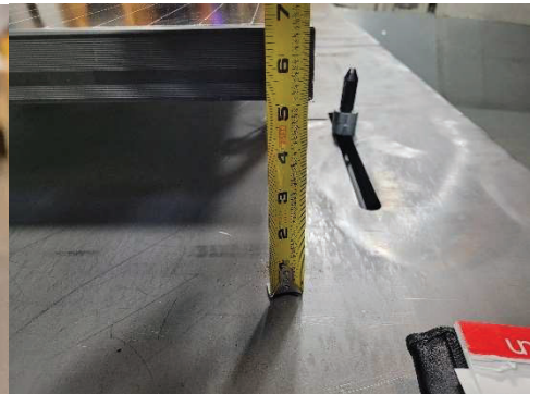
Figure 6: Height from roof to panel, Runs 2 & 3
