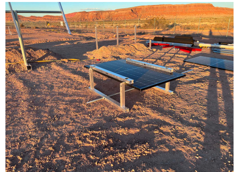
PHOTO 3: IR-30 Solar Racking System setup for test
