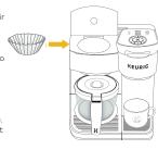
NOTE: The maximum capacity for regular ground coffee is 15 tablespoons and 12 tablespoons for decaf. Exceeding this amount may cause overflow.
