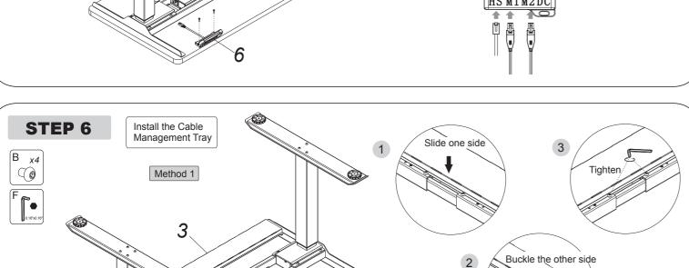
Firstly, rotate the screws (B) incompletely into the supporting beam (4) with Allen Key (F), which means do not tighten them. Next, slide one side of the cable management tray (3) into the screws (B), then the other side Finally, tighten the screws (B) with Allen Key (F).
