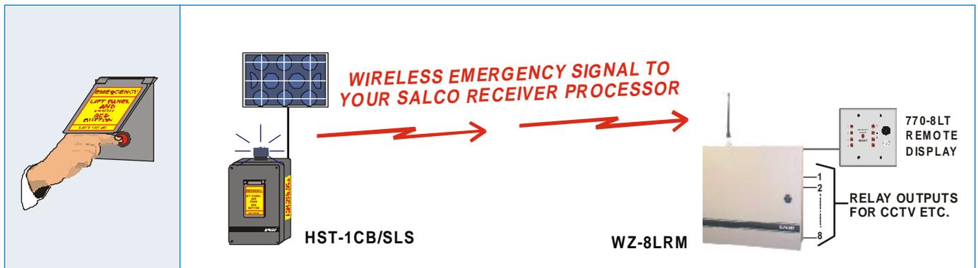
**WIRELESS RECEIVER INTERFACE / EXPANDER / ANNUNCIATOR****WZ-8LRM Wireless Interface System**
