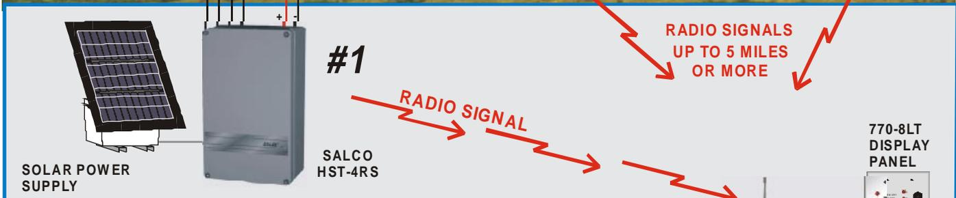
The wireless solar-powered outdoor perimeter fence system transmits a radio signal to the WZ-8LRM receiver processor located up to five miles away, or more with accessories. Each fence system comprises a solar power supply, fence detection processor, and radio telemetry transmitter and can accommodate a linear fence length of 800 to 1000 feet.
